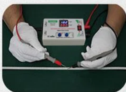
LED single lamp bead reverse test
