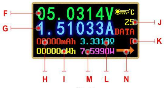
powered on. When the data group 0 is selected, the current value of mAh and mWh will be temporarily saved at power off. When the device is next powered on these values will be recalled and display in blinking. When the accumulated mAh exceeds 1 mAh, the previous data will be cleared and accumulation will restart.
