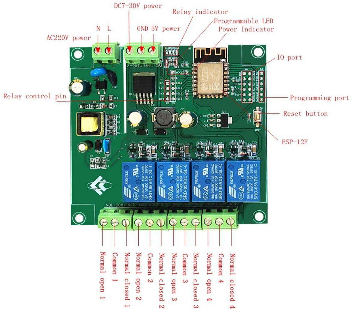
Programming port: ESP8266's GND, RX, TX, 5V are respectively connected to the GND, TX, RX, 5V of the external TTL serial port module. IO0 needs to be connected to GND when downloading, and then disconnect the connection between IO0 and GND after the download is complete;
