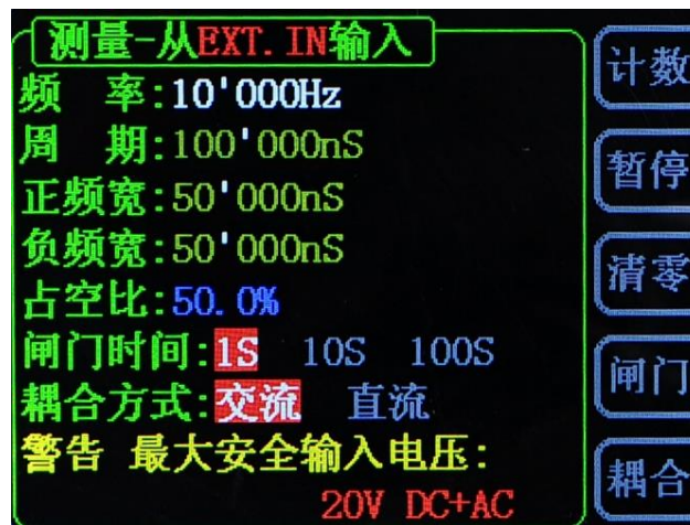
2-1 Frequency meter / counter parameter setting interface
