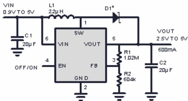
\*LOCATE COMPONENTS CLOSE TO THE PIN
