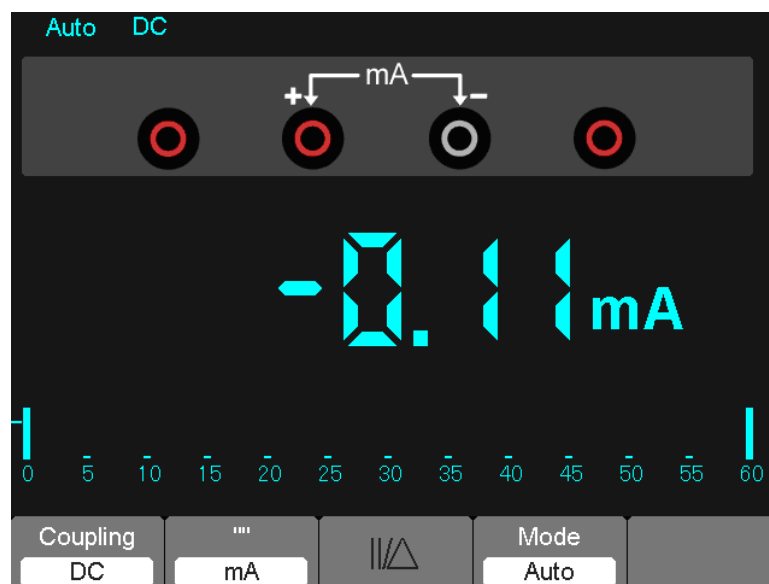
Figure 7-8 DC current Measurement for 600 Measurement
