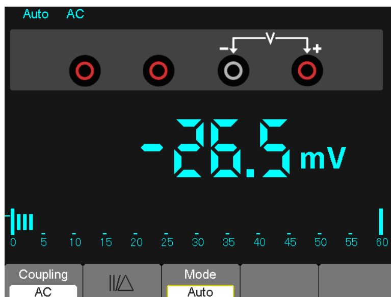
Figure 7-7 AC voltage Measurement
