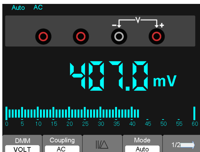
Figure 7-7 AC voltage Measurement
